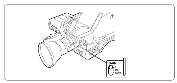
Gain settings of 0/6/12dB or 0/9/18dB are set on the menu item CAMERA SETTING menu screen for operation. (The 0/6/12dB settings were selected when the unit was shipped from the manufacturing plant.) For further details, refer to the menu items (on pages 48, 49 and 53).
